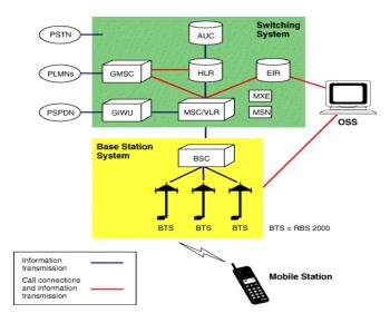
Figure 1: The GSM Network System
